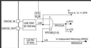
Each clock source can be switched on or off independently when it is not used, to optimize power consumption.
