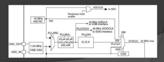
The PLL input clock frequency must be between 2 and 24 MHz.
