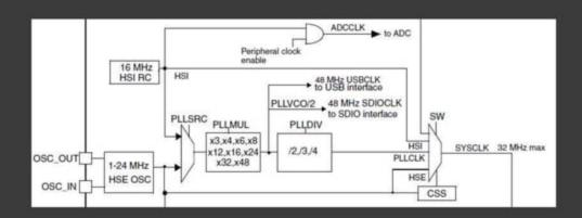
PLL VCO clock (defined byhe PLL multiplication factor) must be programmed to output a 96 MHz frequency.
